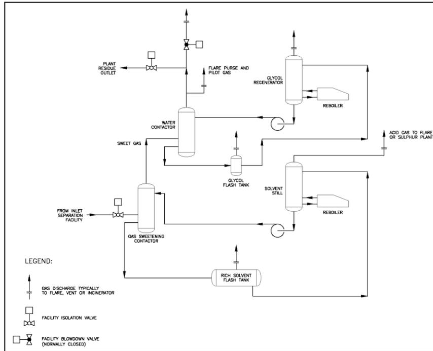
Figure 11.3: Reportable Flaring Streams – Gas Processing Plant
