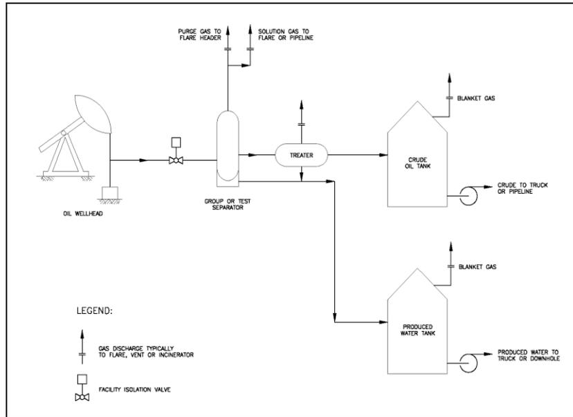
Figure 11.1: Reportable Flaring Streams – Upstream Oil Battery
