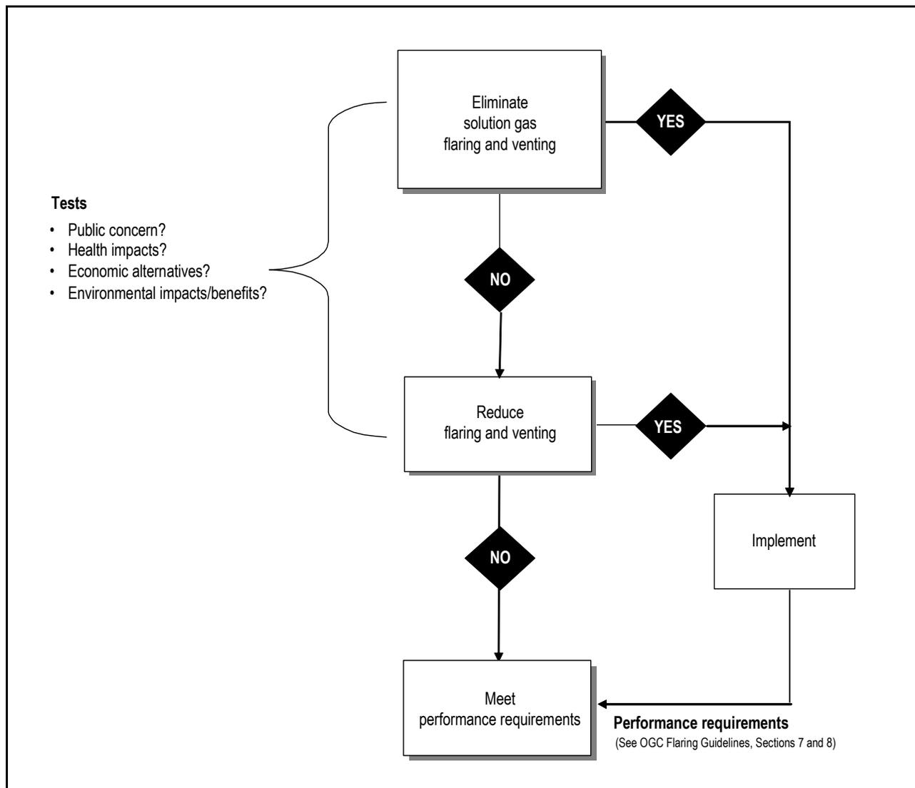
Figure 2.1: Solution Gas Flaring/Venting Decision Tree (adapted from CASA)
