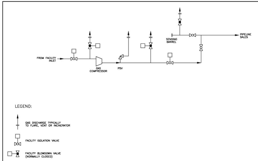
Figure 11.4: Reportable Flaring Streams – Gas Compression Facility
