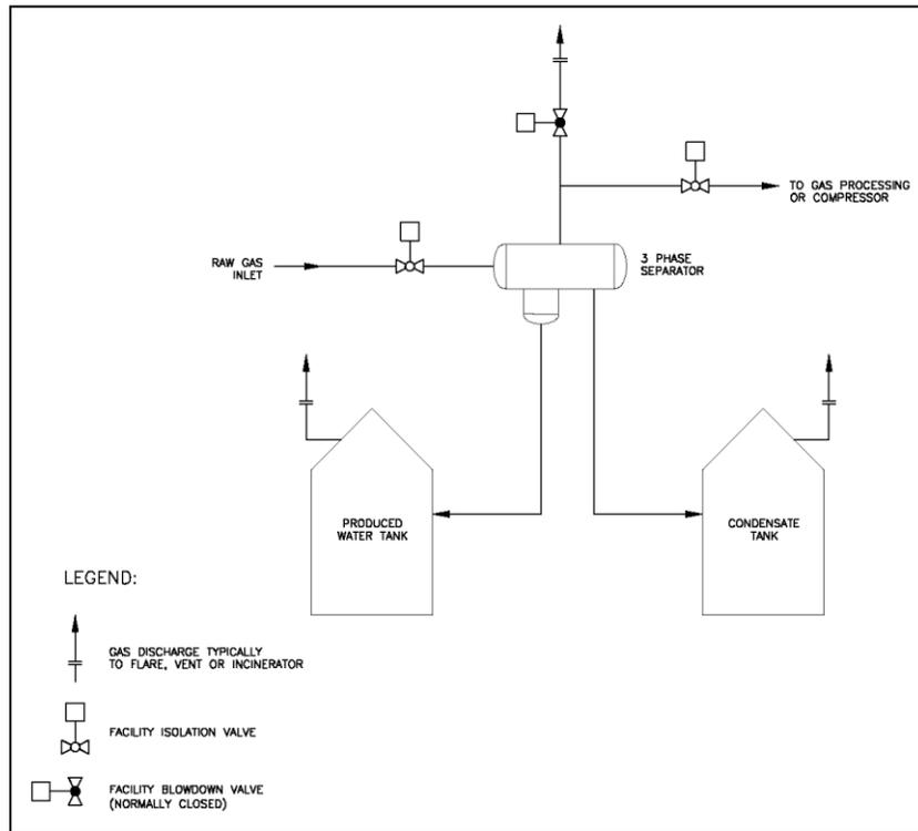
Figure 11.2: Reportable Flaring Streams – Inlet Separation Facility
