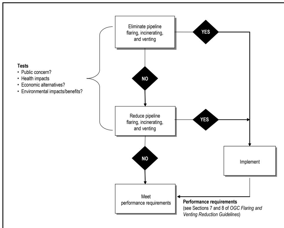
Figure 5.1: Pipeline Flaring and Venting Decision Tree (adapted from CASA)
