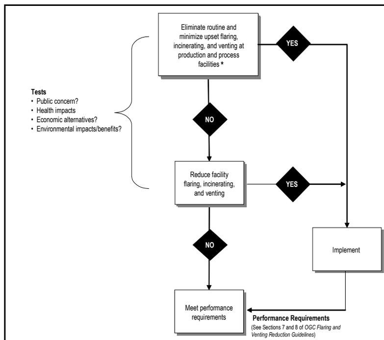
Figure 4.1: Facility flaring and venting decision tree (adapted from CASA)
